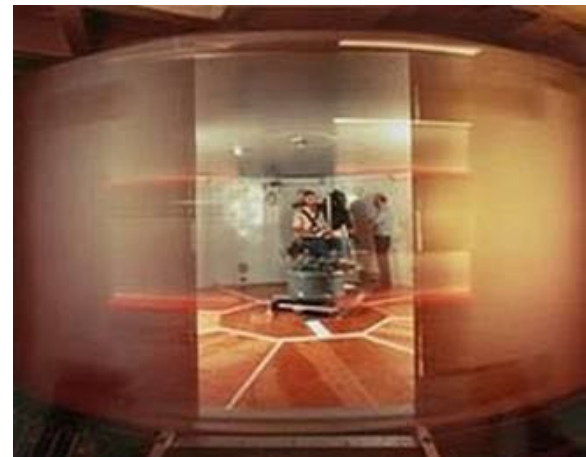
Fig. 3. The experiment set up of the rotating room with the subject sat in the center of rotation.
