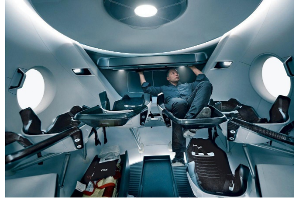
Fig. 11. Mock-up of the crewed dragon. Like the stripped-down version proposed for the testbed. All outfitting will be removed and replaced with an open plan laboratory. Autonomous launch will mean no outfitting such as seats and screens inside.
